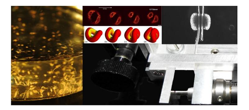
The tissue stretcher  $\mu$ N-TS is designed for characterisation of different tissues types – study of tissue contraction, measurement of forces and structure in the tissue, stimulation by forces, electrical fields and drugs.
