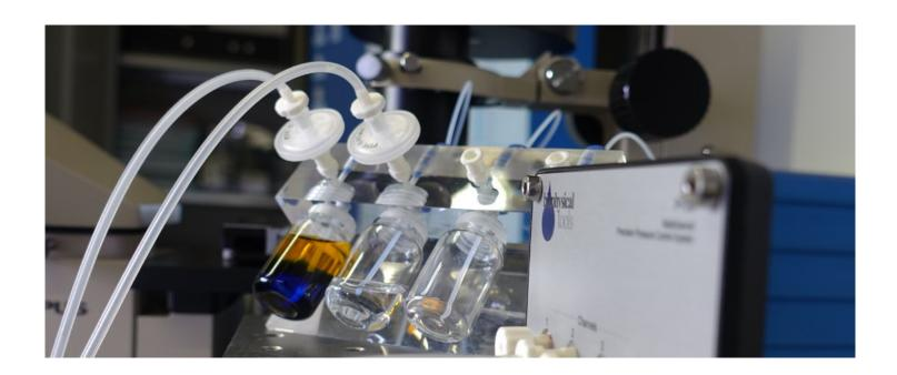
Content Management Unit is designed for a user-friendly storage of reagents and liquids during a microfluidic experiment. Different volumes are available. The content management unit can be used with standard vial threads for the volumes 1.5 mL, 4 mL and 10 mL. CMU has standard threads for connectors: UNF 10-32, compatible with M5. So, you can exchange connectors and fingertight fittings depending on your needs towards tubes.
