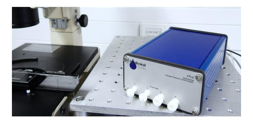
P<sup>2</sup>CS is a precise pressure control system, which provides pnemautic actuation and flow control. It allows a new level of fluidic control in nano-, micro- and mesofluidic channels and capillaries. As it regulates pressure and vacuum, bidirectional fluidic control, fast stopped flow and pulse function realisation become possible. A two-level pressure system with two sensors per channel enables precise control for high and very low flow rates.
