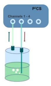
DROPLET GENERATION WITH  $P^2CS$  EVEN JUST IN A Y-SHAPED MICROCHANNEL: USE CONTINUOUS FLOW, OR PULSES, OR THE FUNCTION GENERATOR TO GENERATE DROPLETS
