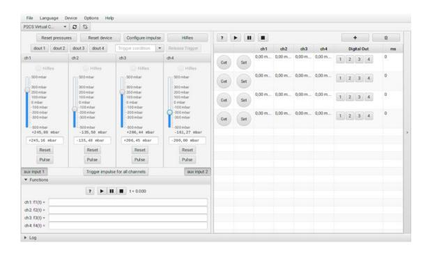
jP<sup>2</sup>CS allows as manual as automated control of the flow in the microfluidic chip. In addition, you can configure pulses and use them for a pre-set period of time in the respective channel.
