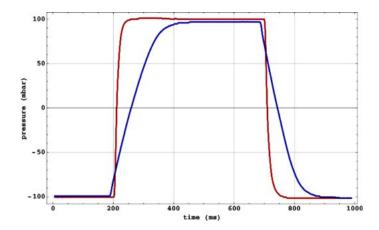
You can run an automatic function for pressure, e.g.  $30 \sin(t)$ . The pressure values follow the graph in real-time on the microcontroller. No additional time is lost, since the function generator is implemented in the hardware, not in the control software on your PC.
