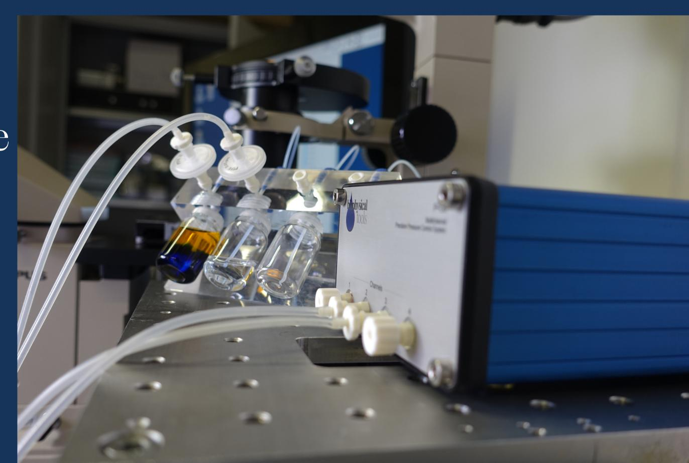
Valve switching unit FS and perfusion head
